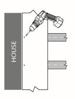
Fasten one edge of the first board at each framing support using a quality 2½" (64mm) deck screw. It is important that this board is straight and well secured.
