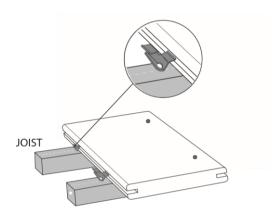
Fully insert TC-G or TC-120 fastener into grooved edge of deck board. Screw hole should line up with the center of support joist.
